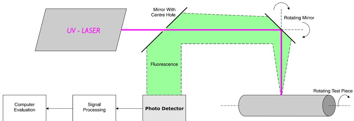
A UV laser beam is directed towards the test piece during testing. The laser beam path passes a number of mirrors that can be moved allowing the test component to be scanned. Please refer to the illustration opposite.
