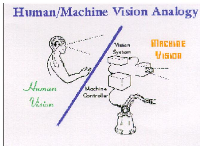
A model of machine vision is quite similar to the simplistic model of the human vision system. A camera with a lens forms the optical image onto an image sensor, a video signal then travels through a cable to a computer that analyses the image information to extract the necessary information. This information is then sent to a controller which operates some machinery.
