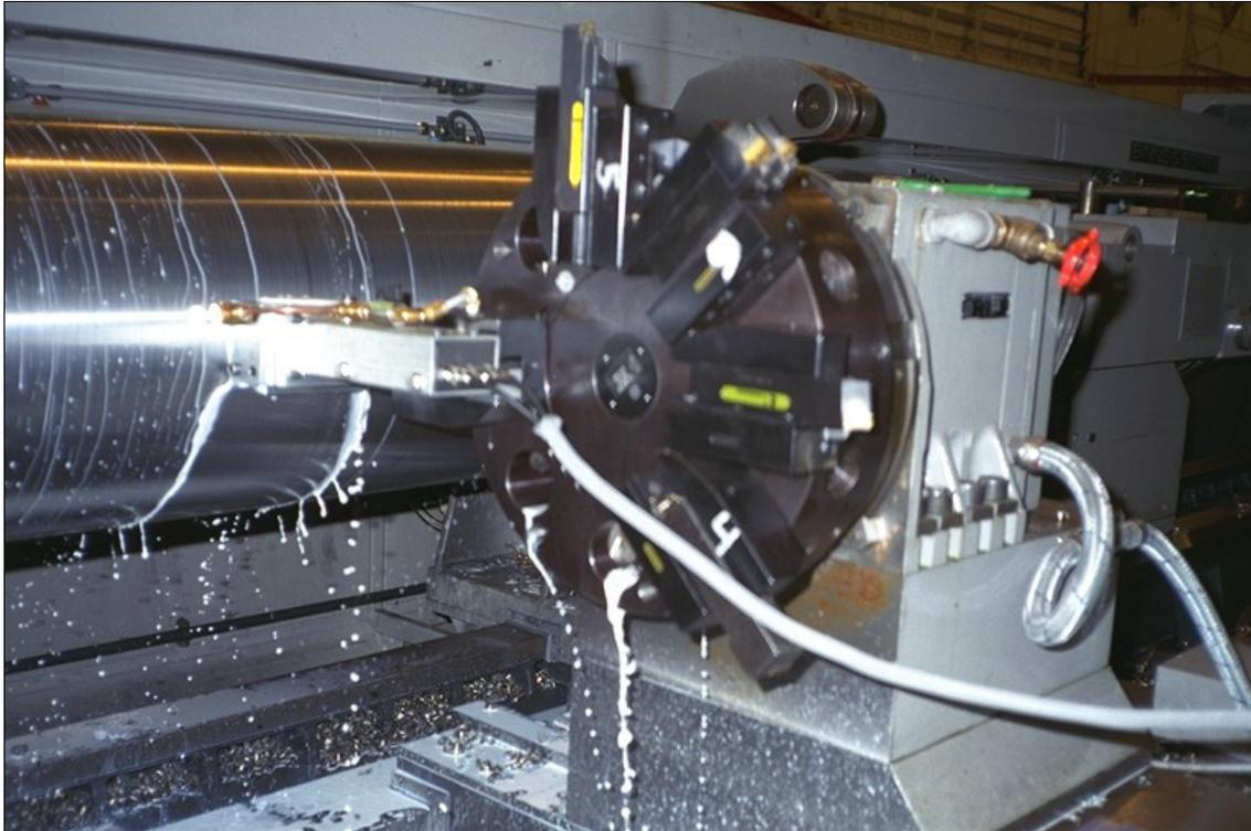
This equipment is for the ultrasonic inspection of cast rolls following a period of service but prior to machining them in a CNC lathe. The ultrasonic inspection is carried out using a single fixed **Water Column Coupled Probe (WCCP)** unit for the longitudinal shear wave flaw detection in both directions. See the reverse of this brochure.
