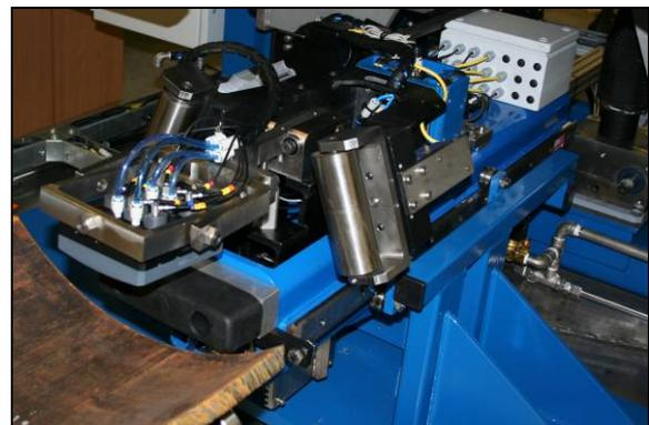
The Ultrasonic system meets the requirements set out in the following Ultrasonic inspection standards; ISO13663:1995(E), ISO11496:1993(E), EN 10246-16:2000 and EN10246-17:2000.
