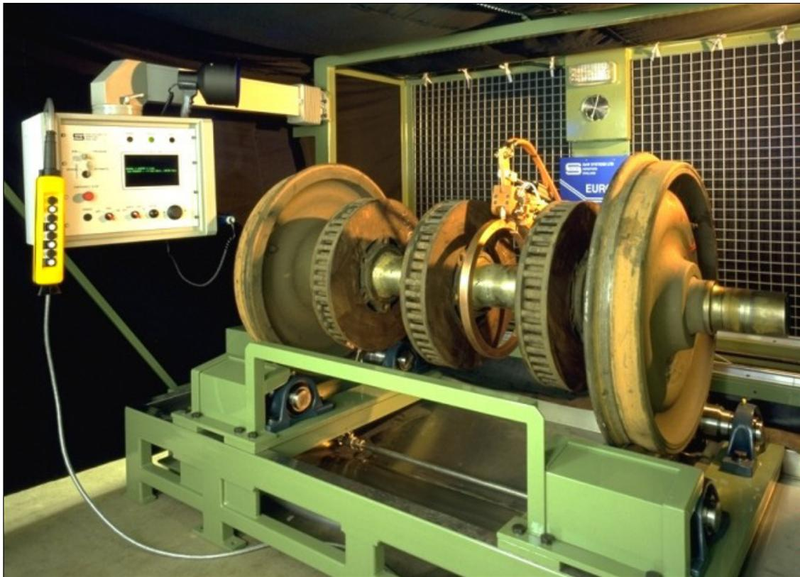
Railway axles which have been in service are routinely tested for surface breaking cracks. One method of testing is the highly sensitive Magnetic Particle Inspection technique which detects any fatigue cracks on the axle. See the reverse of this brochure.
