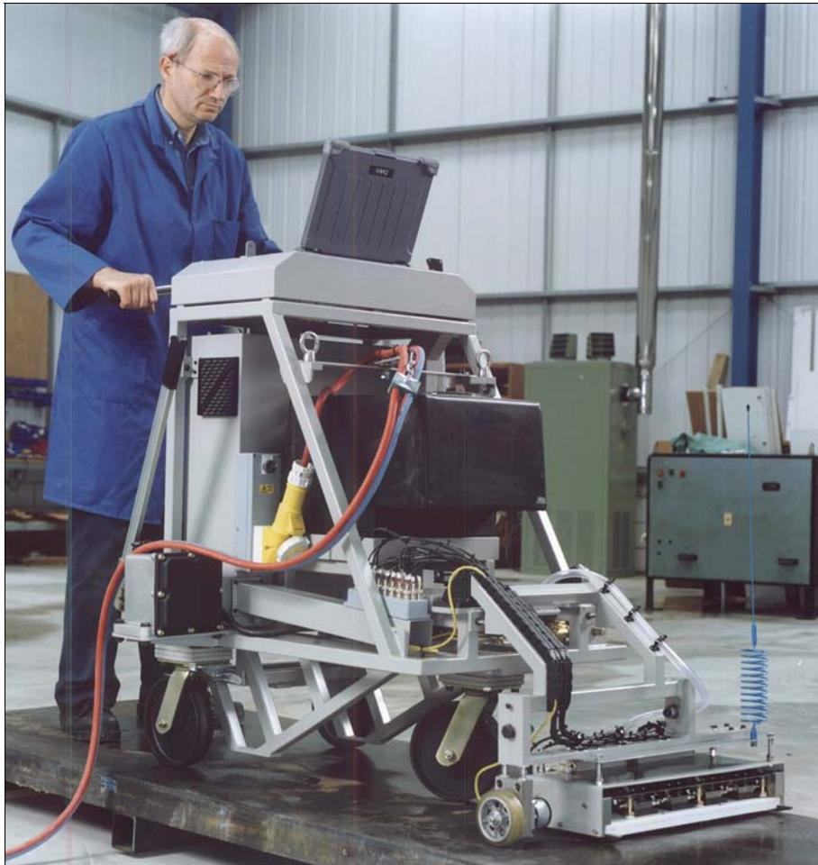
This equipment is a convenient and easily mobile trolley which is manoeuvred around the plate to ultrasonically inspect plate products. See the reverse of this brochure.
