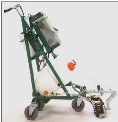
These trollies are pushed over steel plate ensuring the surface area is completely covered, while, the ultrasonic system monitors the signal from the transducers in
