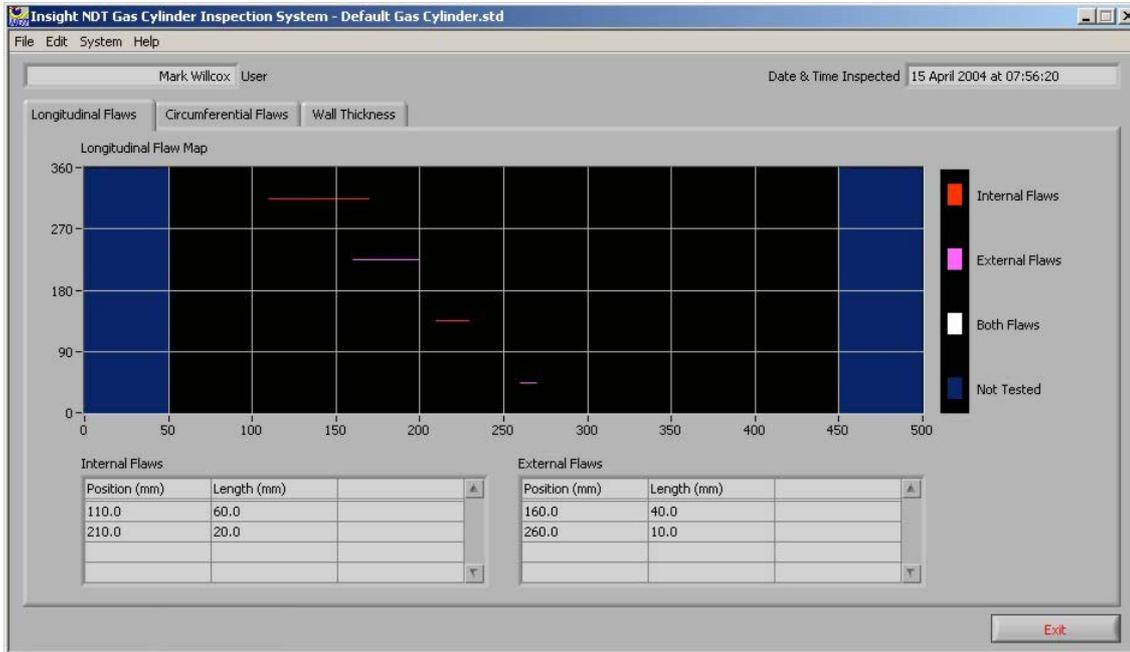
This gas cylinder software has been specifically designed for Ultrasonic Inspection of seamless gas cylinders to BS5045, EN1964 and ISO11439 on a 100% inspection basis.
