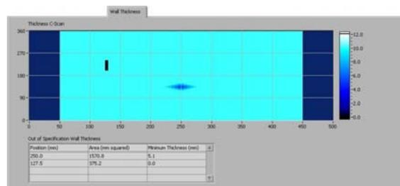
The flaws are represented graphically on the chart. In addition to this chart, there is a single text control which displays the area, position and minimum thickness of the wall thickness flaws found.
