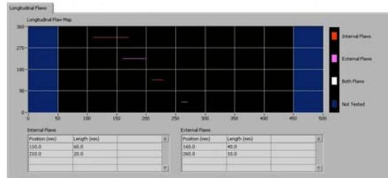
The flaws are represented graphically on the chart. In addition to this chart, there are two text controls which display the position and length of flaws found for both internal and external flaws.
