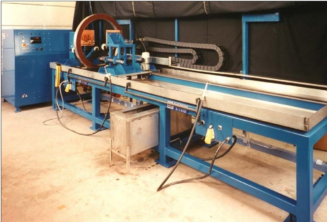
This equipment is for the magnetic particle inspection of large aerospace components such as engine shafts. The machine provides motion control of the coil and the tailstock, thus ensuring a quick and easy set-up from component to component. These features are programmable, thus further reducing the change over time for any given component. See the reverse of this brochure.
