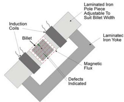
Each yoke magnetises two opposite faces by generating A.C. flux between the pole piece ends.
