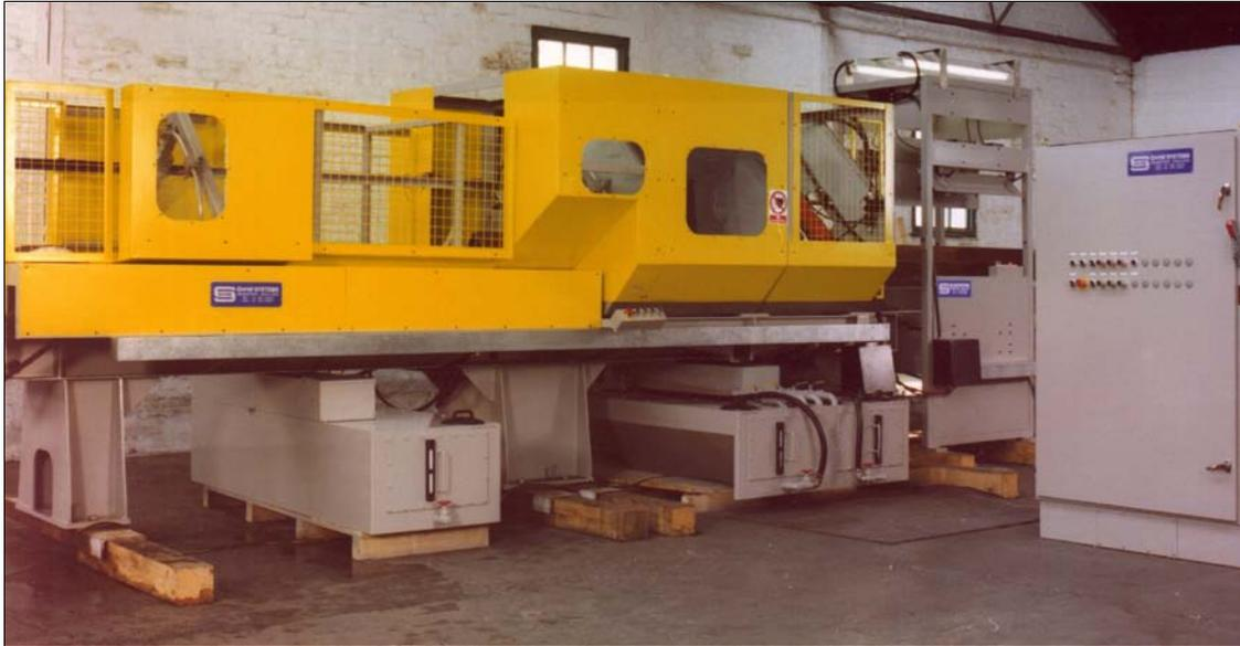
This equipment is specifically for use in detecting surface and near surface discontinuities in ferrous billets of sizes from 120mm square to 200mm square, using a non-contact magnetic particle inspection method. See the reverse of this brochure.
