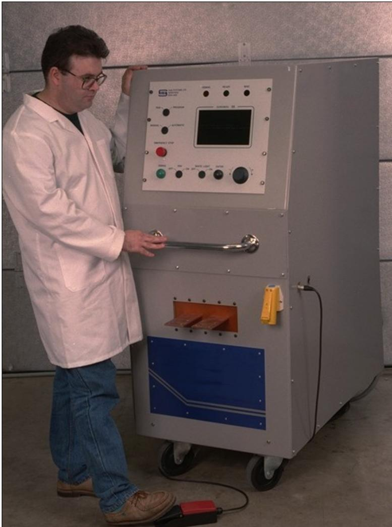
Our power packs are for supplying the high currents required for magnetic particle inspection equipment. See the reverse of this brochure.
