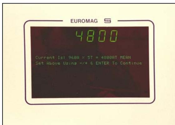
Control of the power pack is through the screen dialogue and simple rotary control and "ENTER" button. The active unit settings are displayed on the screen which also incorporates a large digital ammeter with reading hold facility.
