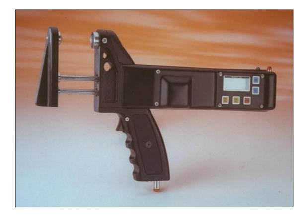
**QUALIRON** consists of a hand held caliper/electronic unit fitted with a display giving velocity readings and acceptance band indicator lamps. The caliper is of lightweight durable construction, well balanced to reduce operator fatigue and allow accurate operation by relatively unskilled personnel. The operator simply places the caliper jaws over a suitable part of the casting and presses the trigger.
